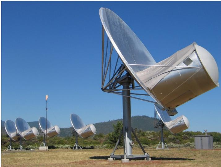
Collaboration with the US Technology Development Program led to the integration of the rim supported concept used in the ATA antennas with the single piece composite reflector surface. The result is the Single-piece, Rim-supported Composite (SRC) Reflector concept.
