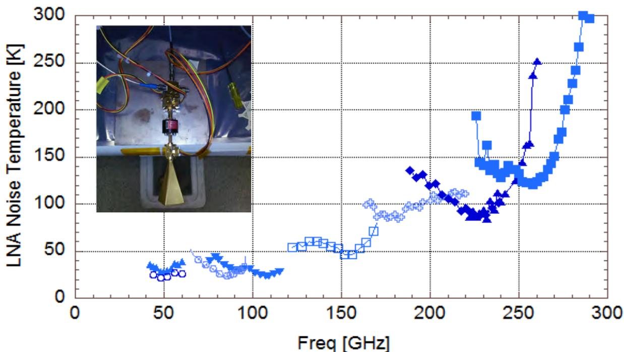
**Measured results for 35 nm InP HEMT MMICs (NGC) over 40-300 GHz, with record noise temperature throughout**
