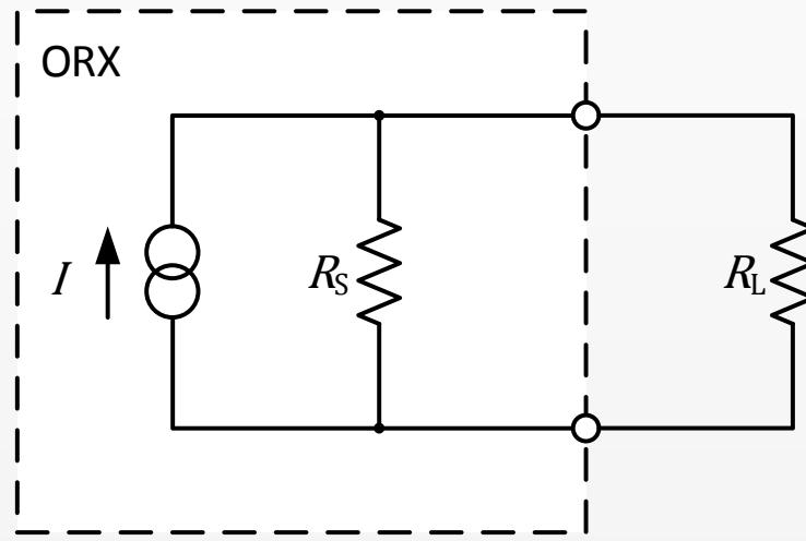
intrinsic photodiode impedance
