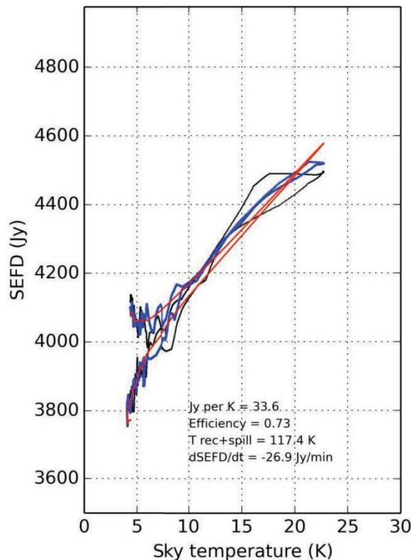
$$SEFD = \frac{2k}{\eta A} (T_{\text{rec}} + T_{\text{spill}} + T_{\text{sky}})$$
