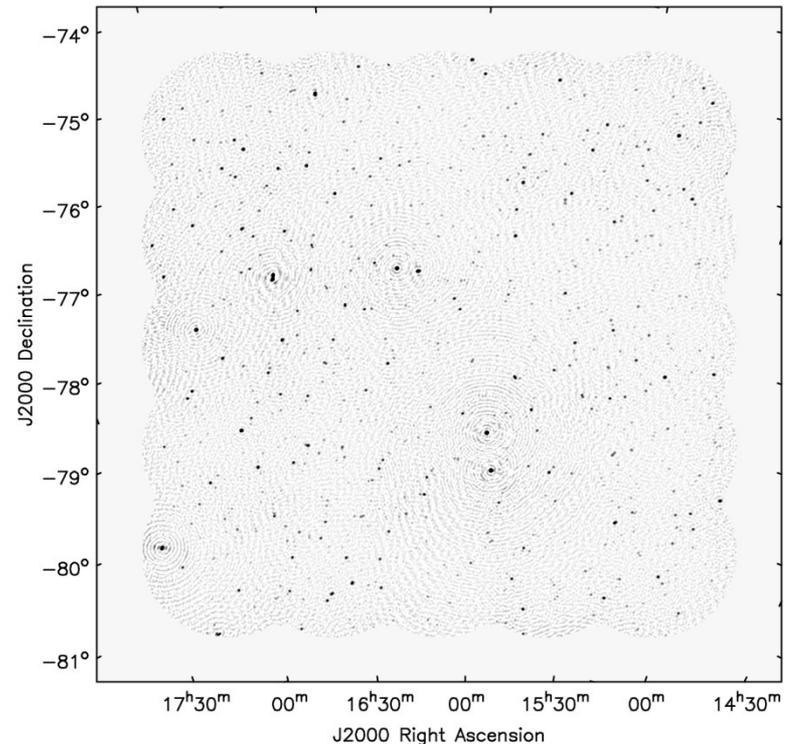
The first ever 25 beam image produced in radio astronomy, using five ASKAP antennas installed with Mk II PAFs at the MRO. This image is approximately 30 square degrees - the complete ASKAP field-of-view. Credit: CSIRO ACES team.
