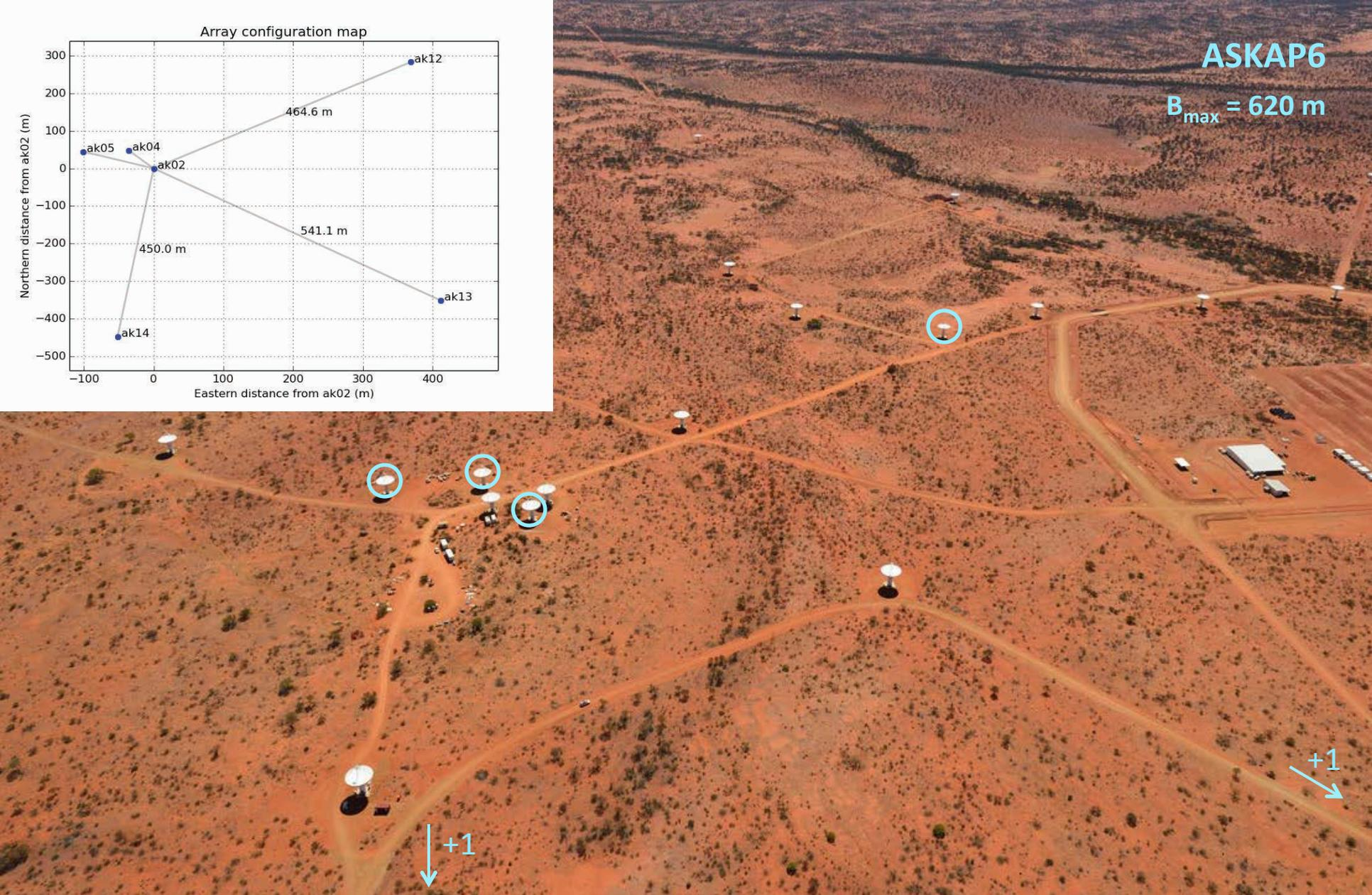
ASKAP6: First 6 ASKAP Antennas with Mk II PAFs | 36 beams
